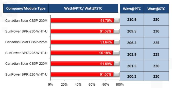
PTC(PVUSA Test Conditions): 1000 W/m2, 20 degrees C air temperature, and wind speed of 1m/s at 10 meters above ground level.
