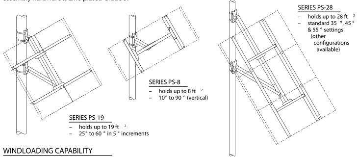
Standard models are designed and warranteed to withstand windloads of 30 lbs./ft mately 90 mph). Designs capable of withstanding greater loads are available for high-wind areas. <sup>2</sup> (approxi-
