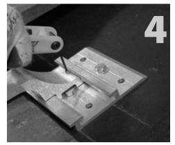
Slide hook into position on base plate. The hook must not overhang the side edges of the base plate. Tighten set screw with hex key.
